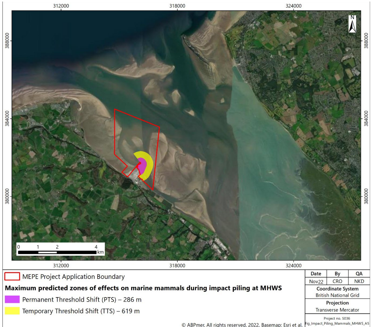
Figure 7. Maximum predicted zone of instantaneous injury and behavioural effects on marine mammals (harbour porpoise) during impact piling at MHWS
