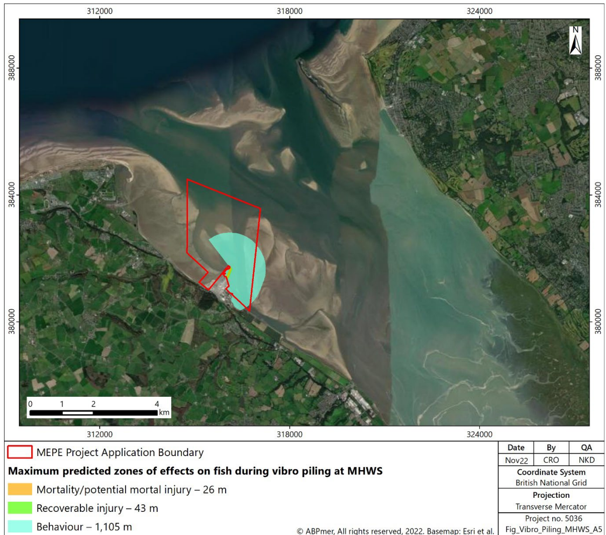
Figure 5. Maximum predicted zone of injury and behavioural effects on fish during vibro piling at MHWS
