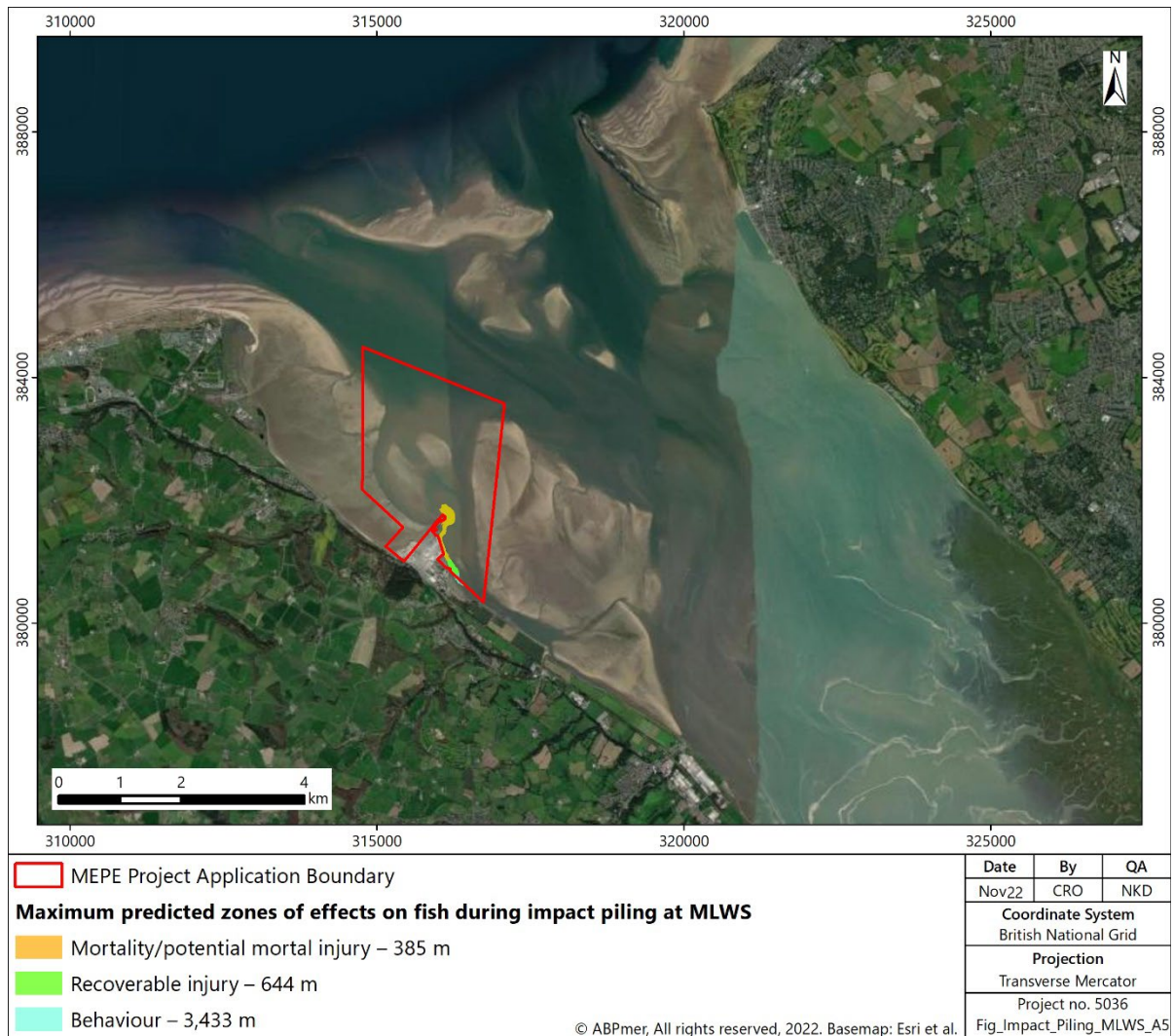
Figure 4. Maximum predicted zone of injury and behavioural effects on fish during impact piling at MLWS
