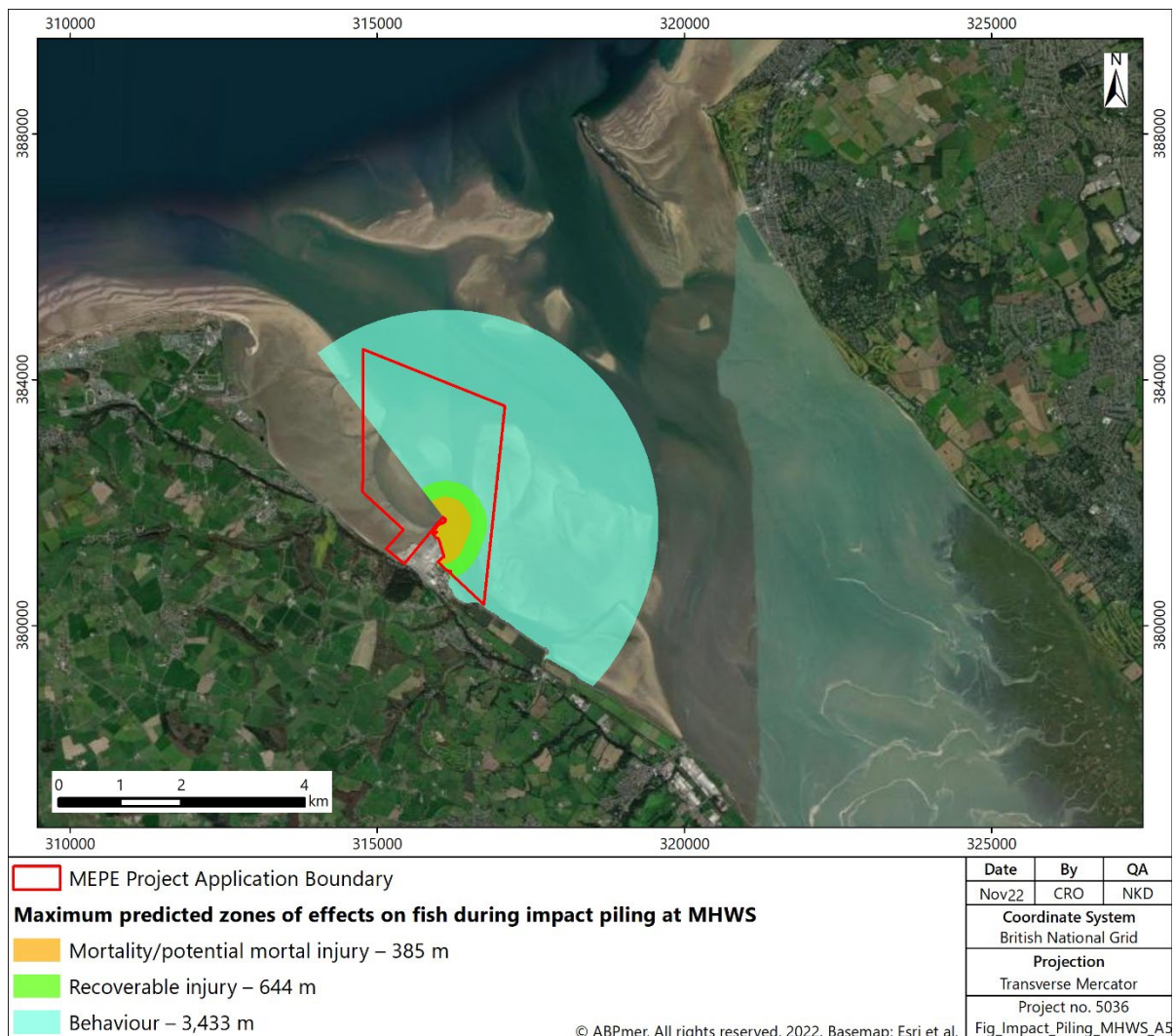
Figure 3. Maximum predicted zone of injury and behavioural effects on fish during impact piling at MHWS
