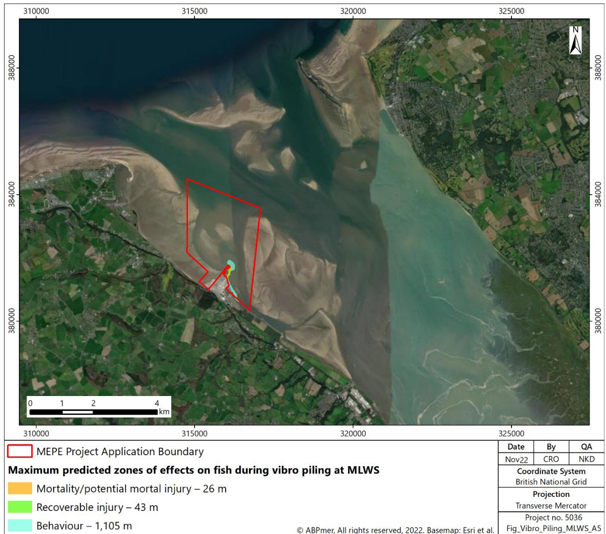
Figure 6. Maximum predicted zone of injury and behavioural effects on fish during vibro piling at MLWS
