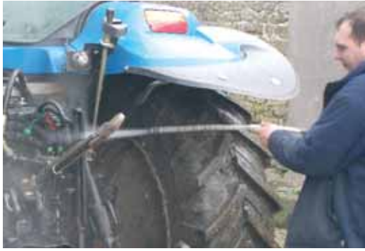
Pressure washers typically use only 8 to 12 litres/min.
