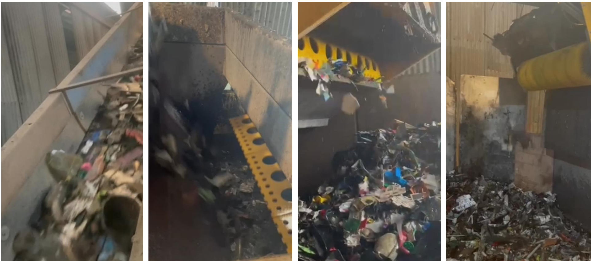
Plate 4-2 Existing sink / float from left to right: (1) conveyor feed, (2) paddle pull into tank and plastic separation output (3 & 4)
