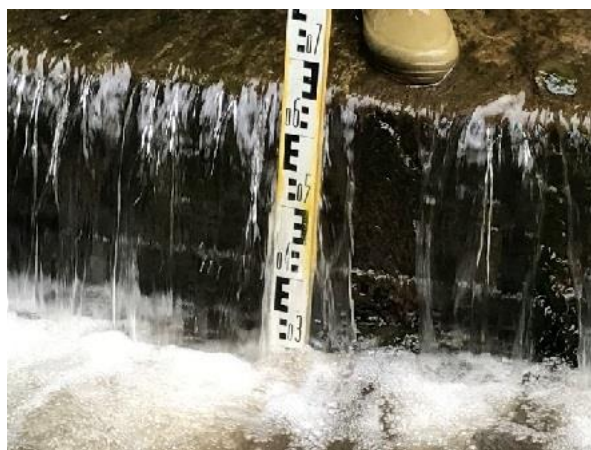
Plate 6-8. Level measurement downstream of the ford (also showing depth of structure)
