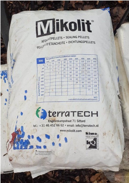
Photograph 2 Bentonite pellets supplied for the works
