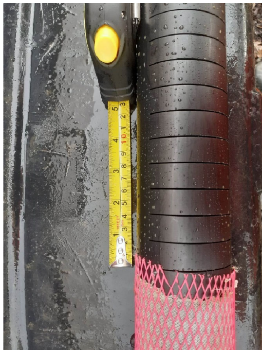
Photograph 4 63mm outer diameter 51mm internal diameter slotted HDPE pipe with Geowrap Geofilter permeable filter geotextile sleeve
