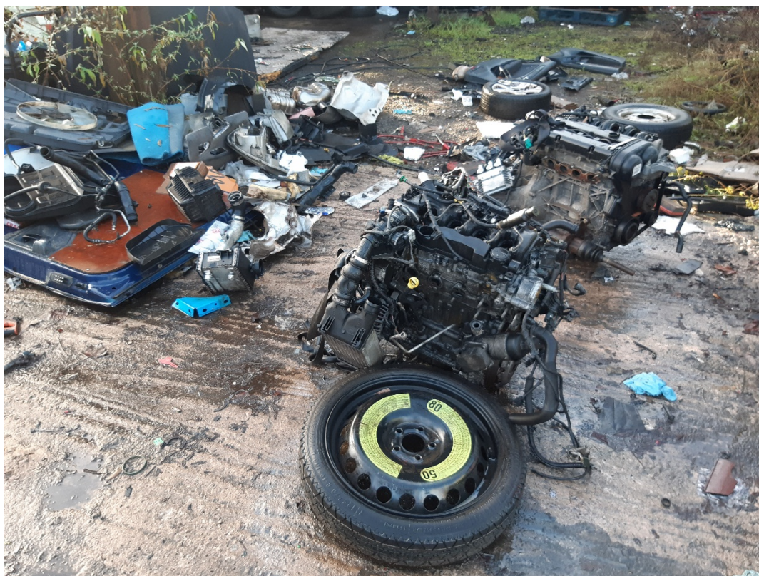
Photo 3 – hazardous wastes stored outside building with oil residues visible on hardstanding
