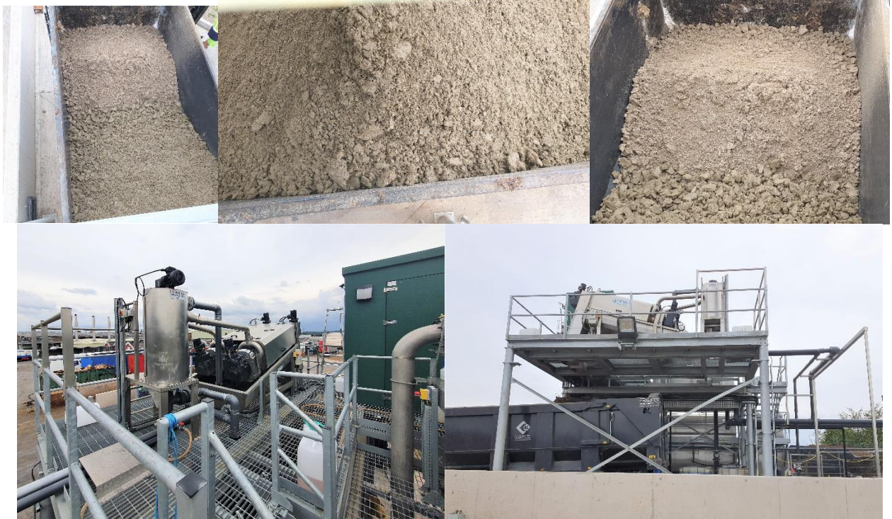
Double Hydro 400 Screw Press on high level platform ABP Shrewsbury
