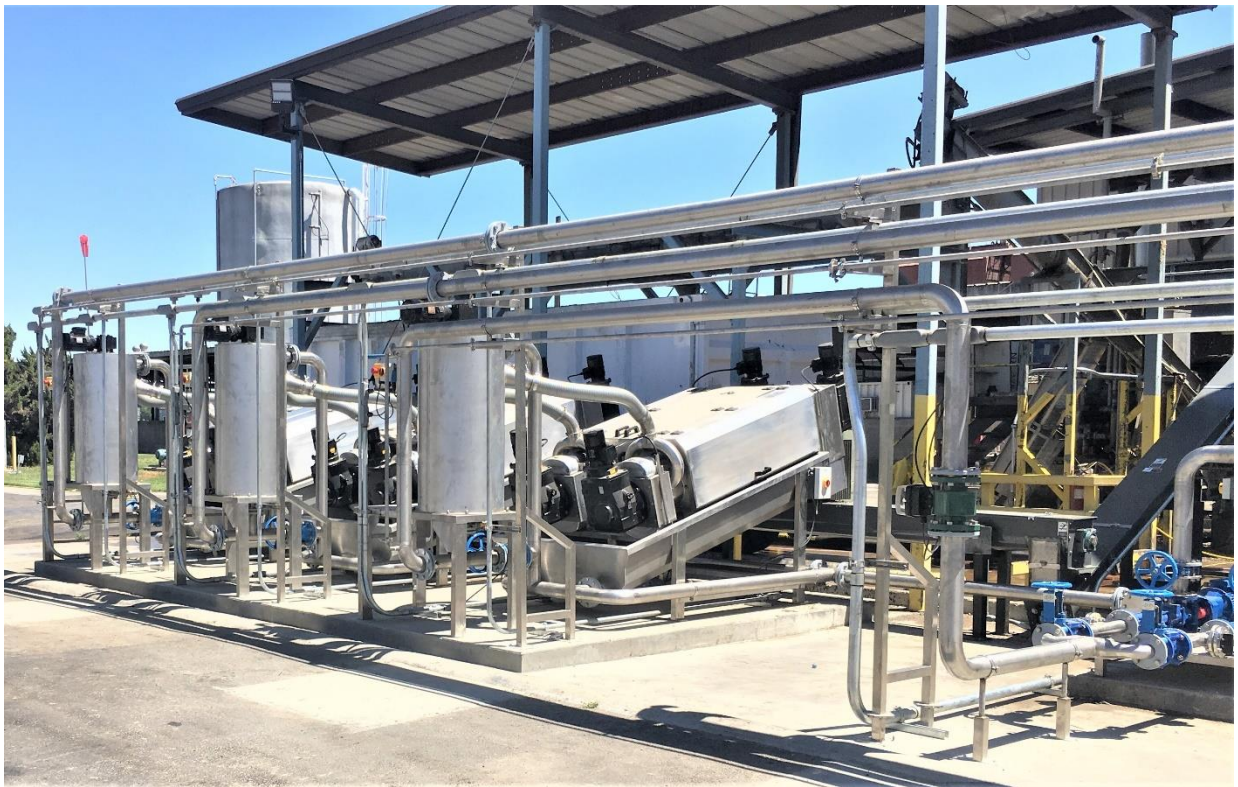
Foster Farms, California, USA, 3No. Hydro Double 400 Screw Press mounted at low level discharging into a common Screw Auger
