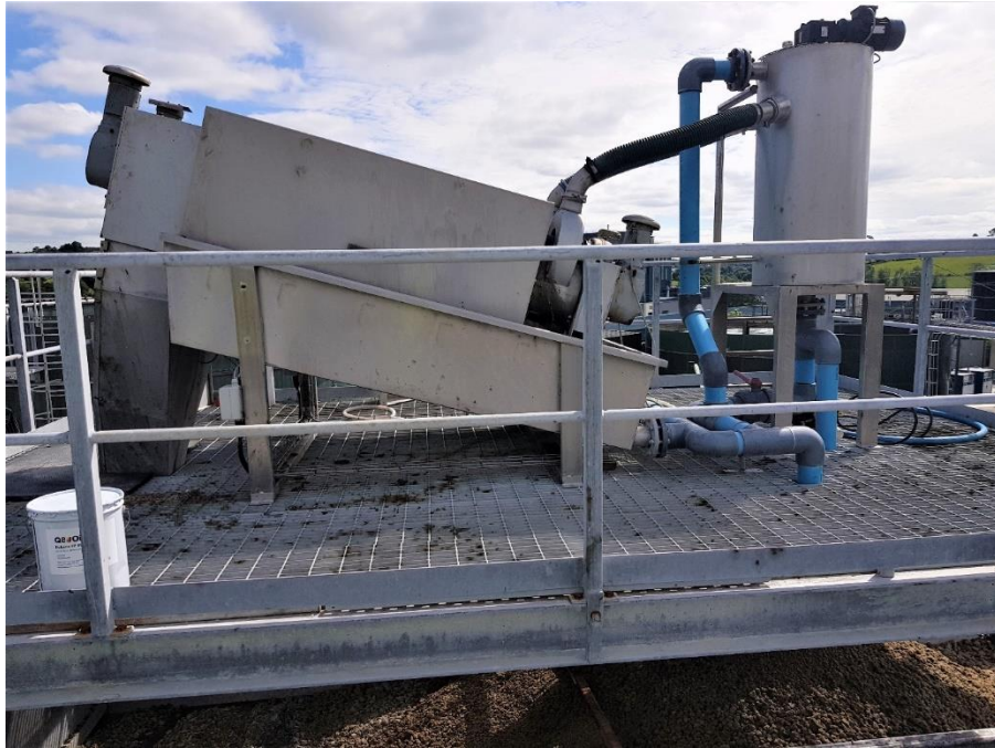
Lakeland Dairies Bailieborough Hydro Double 400 Screw Press mounted on high level platform
