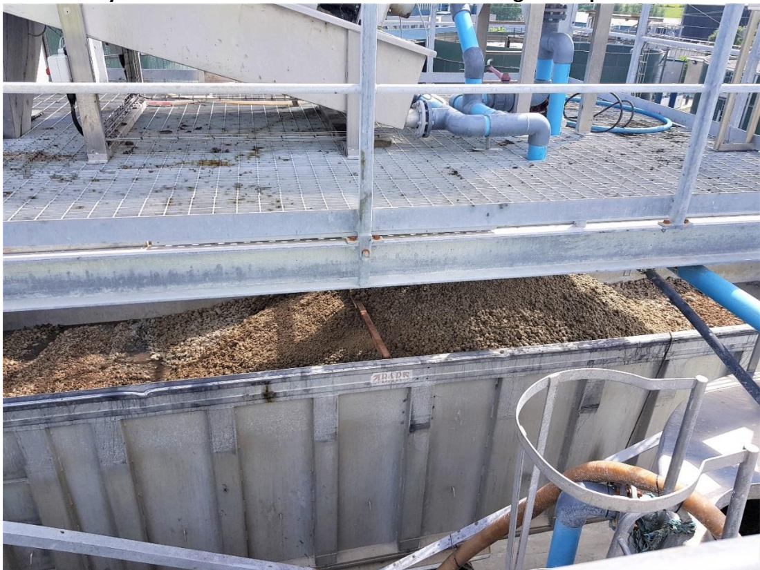
Lakeland Dairies Bailieborough Hydro Double 400 Screw Press mounted on high level platform
