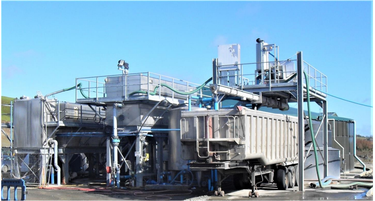
Lakeland Dairies Baillieborough Hydro Double 400 Screw Press mounted on high level platform
