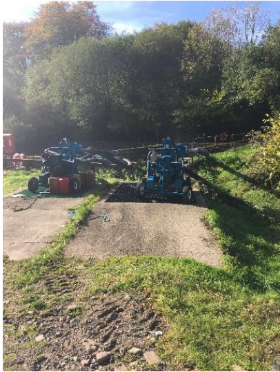
Existing diesel pumps at leachate pond
