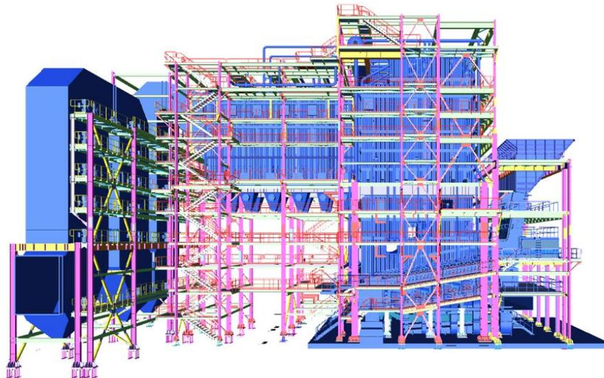
The boiler will comply with the minimum 2 seconds at  $>850\text{ }^{\circ}\text{C}$  residence time requirements under all boiler operation conditions included in the full extent of the firing diagram. The boiler tube panel walls for the first two vertical passes will include multiple openings for thermal temperature mapping instruments to be fitted to enable proof of this requirement, with velocity and residence time being calculated from the boiler thermal design model.
