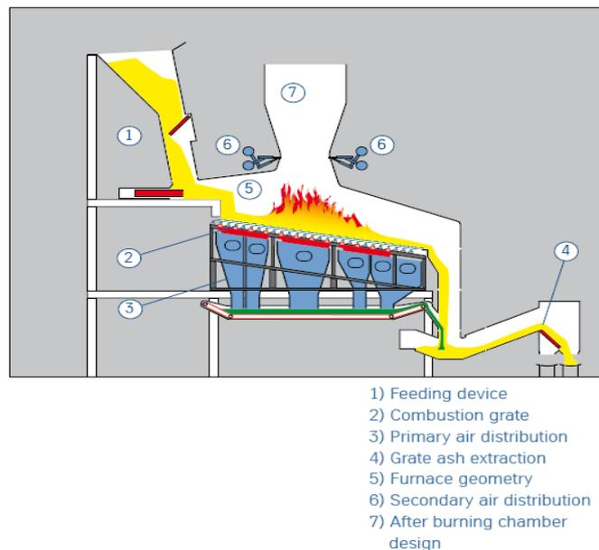
**Figure Grate Firing System (schematic)**
