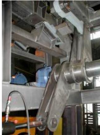
Figure Typical MHPS Hydraulics Grate Drive Arrangement
