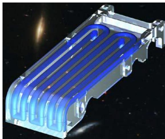
Figure Grate Bar (typical water-cooled design)
