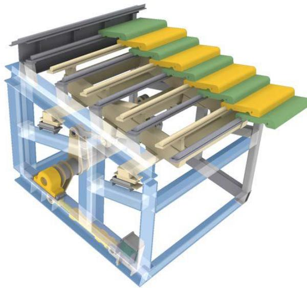
Figure Grate Firing System
