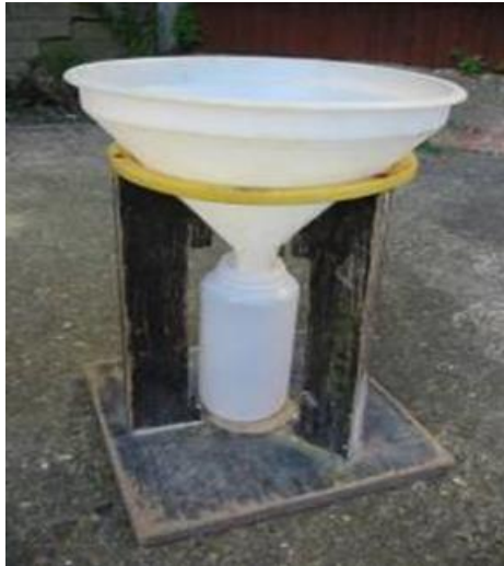
Figure 11. Funnel and stand to assist in the transfer of the biological sample into the sample container.
