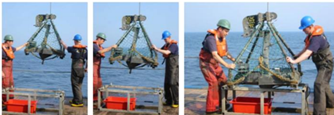
Figure 8. Deployment and recovery of the 0.1 m² Hamon grab.
