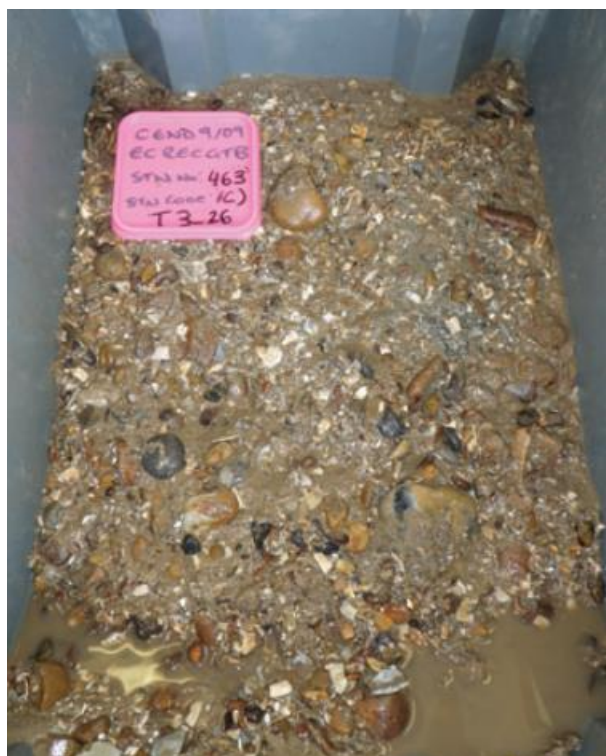
Figure 9. Photograph of 0.1 m 2 Hamon grab sample, including meta-data label (Tupperware lid) taken prior to processing.
