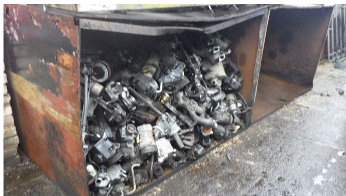
oily parts stored outdoors with no cover
