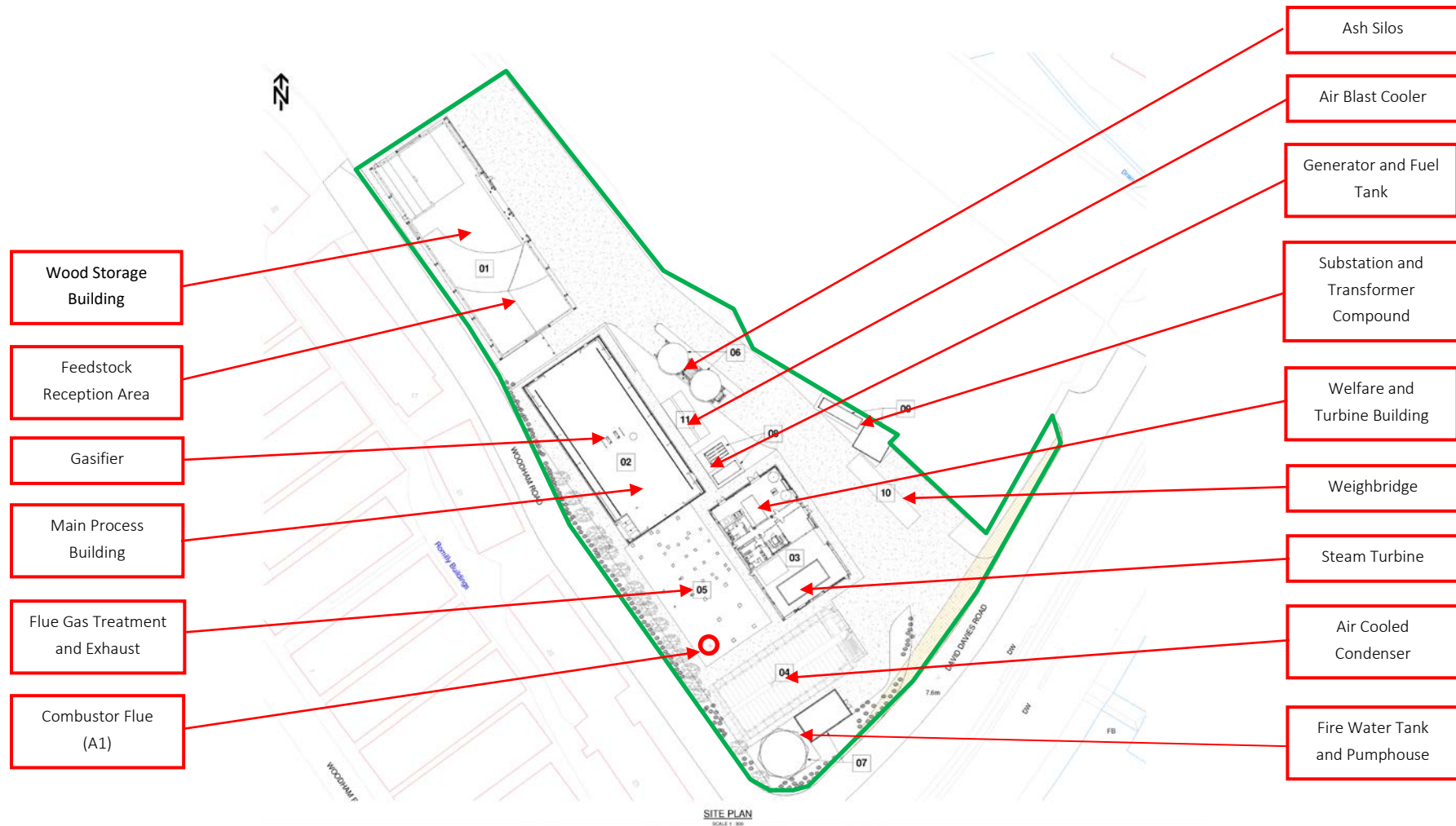
Figure 1.2: Site Plan Showing the Installation Boundary and Key Process Locations
