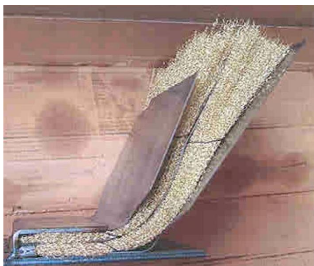
Figure 11: Picture of Tail Skin Sealing Element
