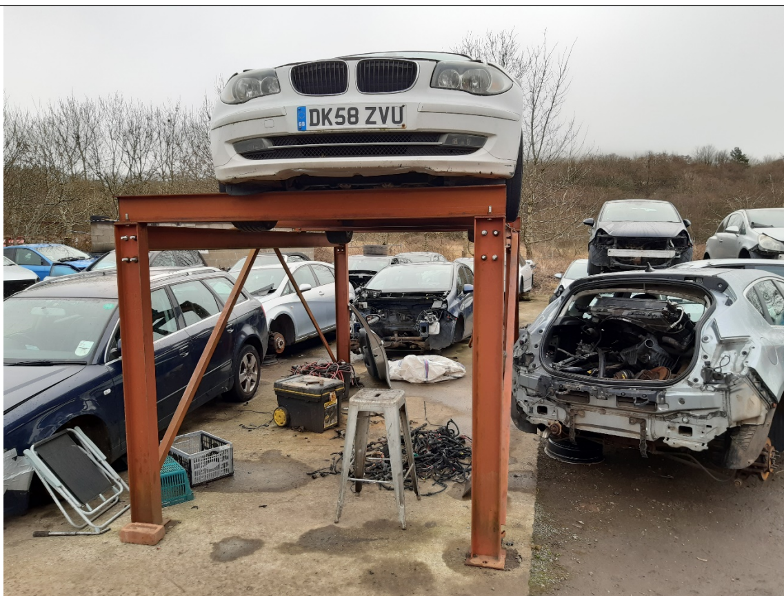
Photo 3 – vehicle awaiting depollution on inspection ramps
