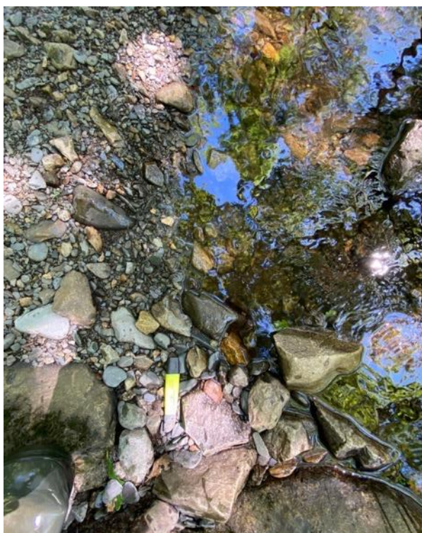
Bed Material (100mm pen for scale)
