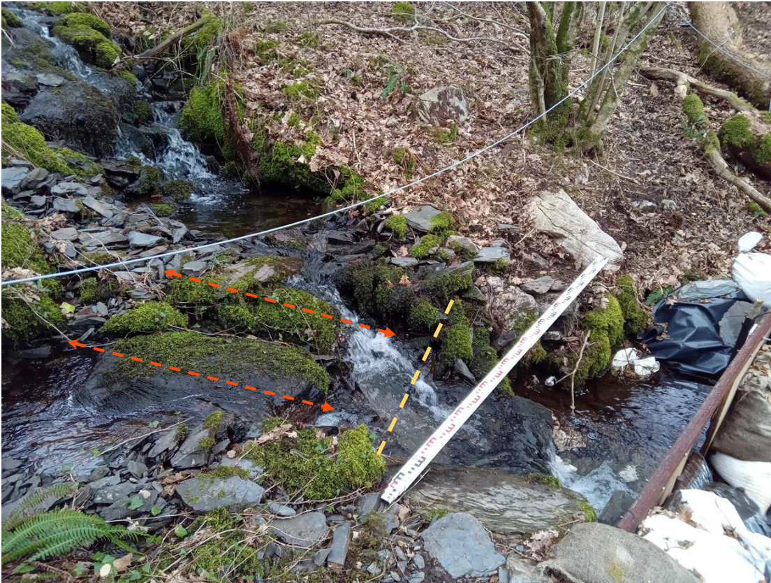
13. Grid Reference: SH 58005 42080 Weir located at natural fall in watercourse in order to create limited impoundment volume (shown with orange arrows)
