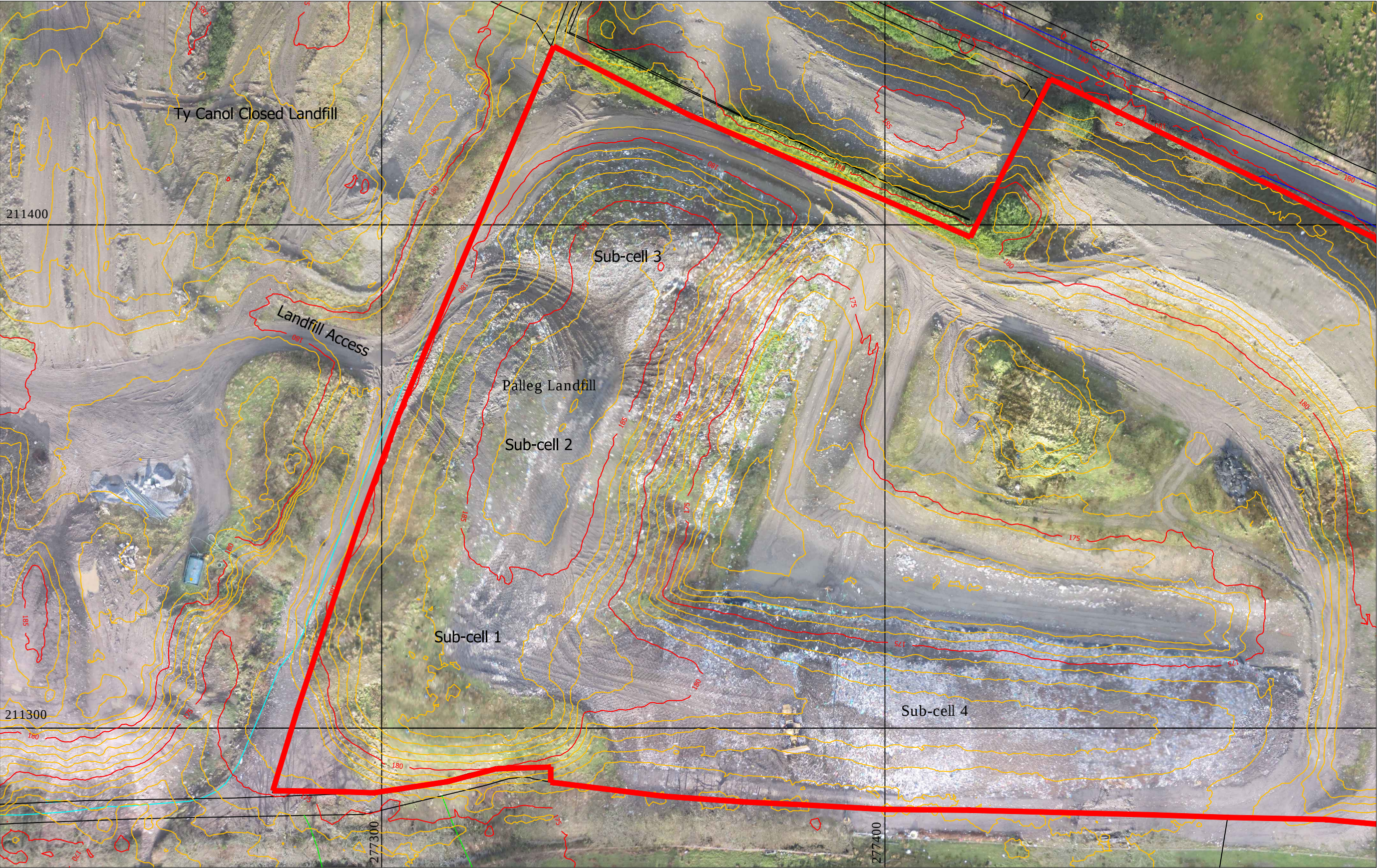
Figure 9 Topographic Survey of Landfill on 6 December 2015 with Aerial Image
