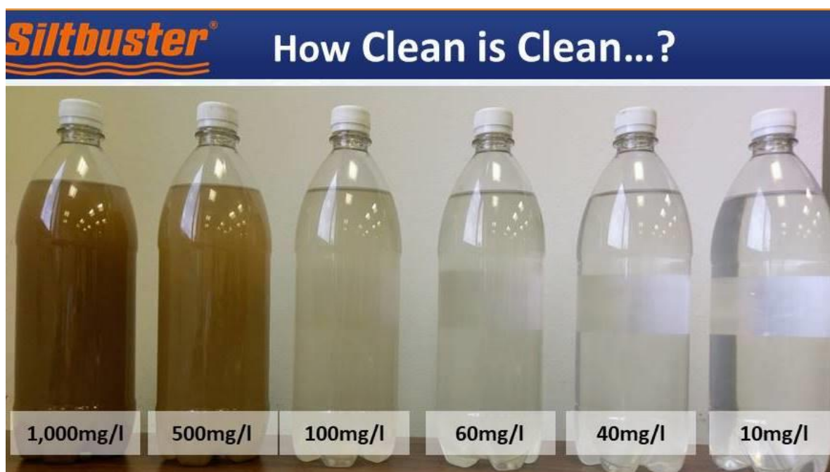
CLAY particles suspended in water at different TSS concentrations
