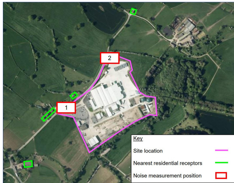
Figure 3.1: Previous noise survey measurement positions.
