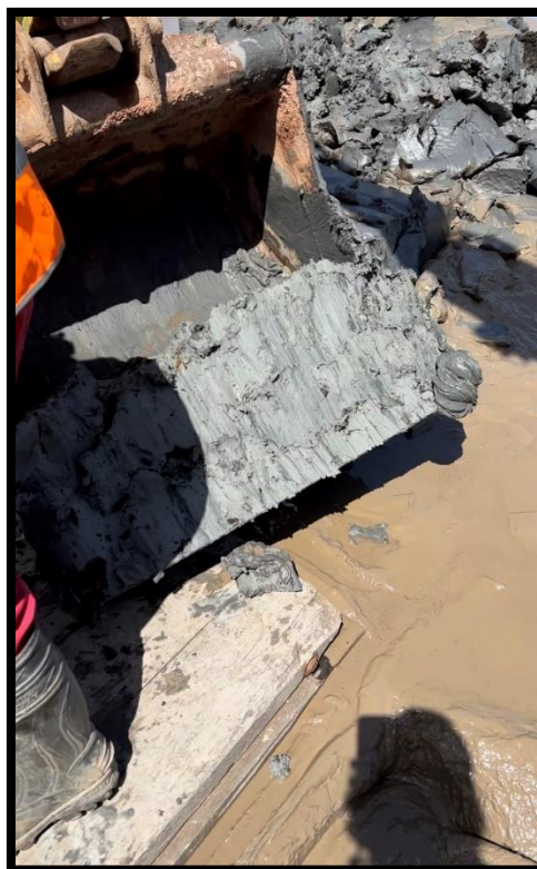
Photograph 11 – Taken during the Ground Investigation works- again, note the consistency of the underlying clay.
