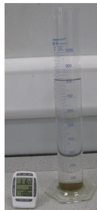
Plate 6: Shaft Settling only 60mins
