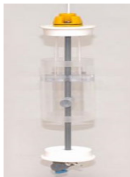
Figure 13 Kemmerer water sampler, used to sample the flooded raise in the drainage adit
