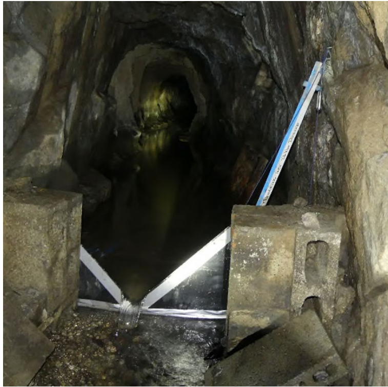
Figure 5 First internal v-notch weir, monitoring the net discharge flow from the mine.
