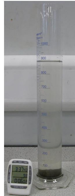
Plate 6: Shaft Settling only 60mins
