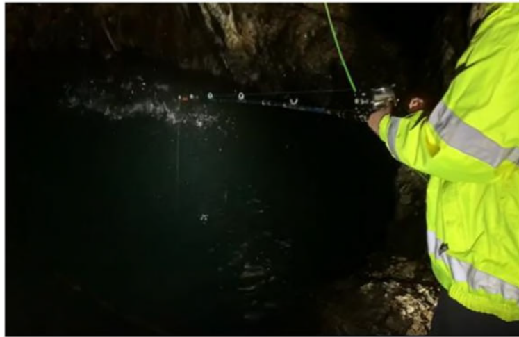
Figure 14 Lowering the Van Essen CTD diver with a fish rod in the flooded Main Shaft from the Llechfraith Drainage Adit, No 2 Level
