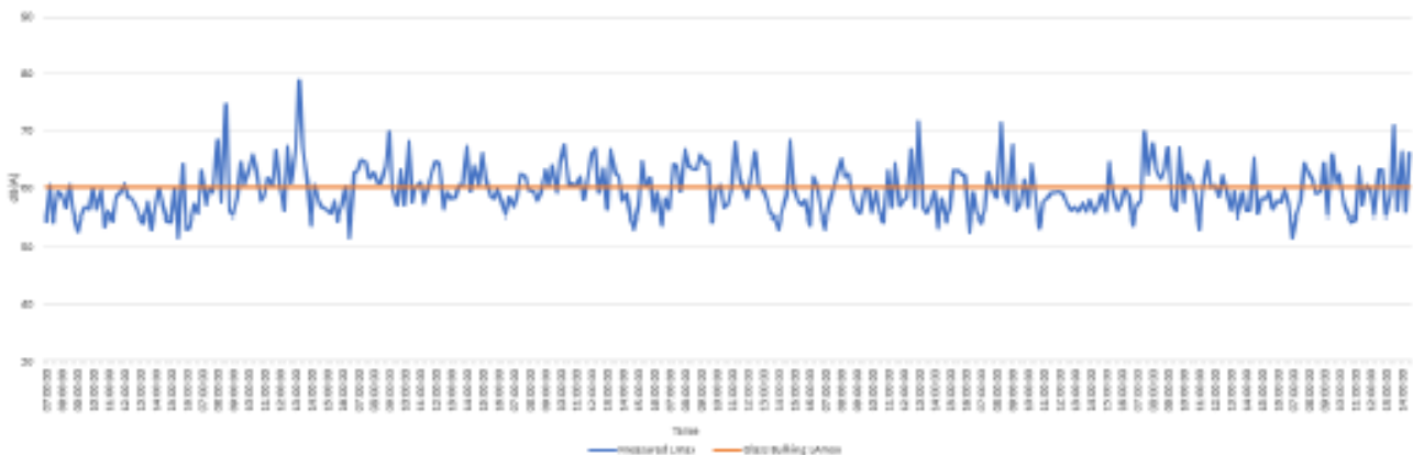
Figure 3: Comparison of Measured Baseline L_{Amax} and Predicted Glass Bulking L_{Amax} Sound Levels at NSR05
