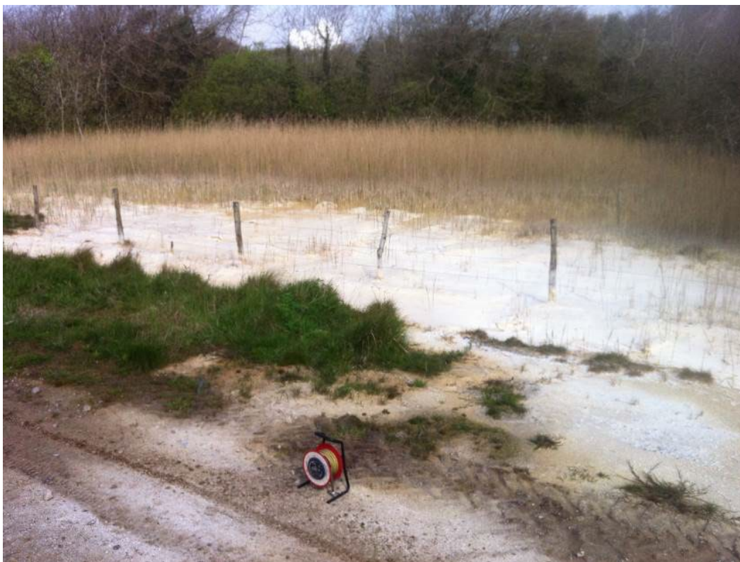
Plate 4-3 Accumulation of secondary precipitates adjacent to MCL (between BH17 and P12)
