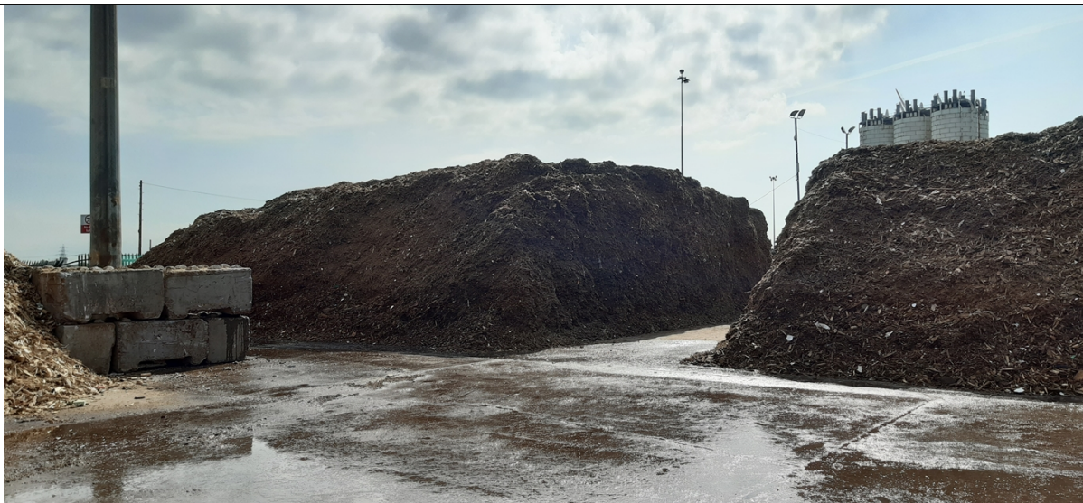
Photo 3 - SWWP Ltd with sufficient fire breaks in place
