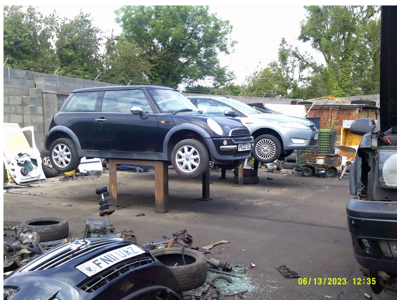
Figure 3: Vehicles on the impermeable surface of the depollution yard.
