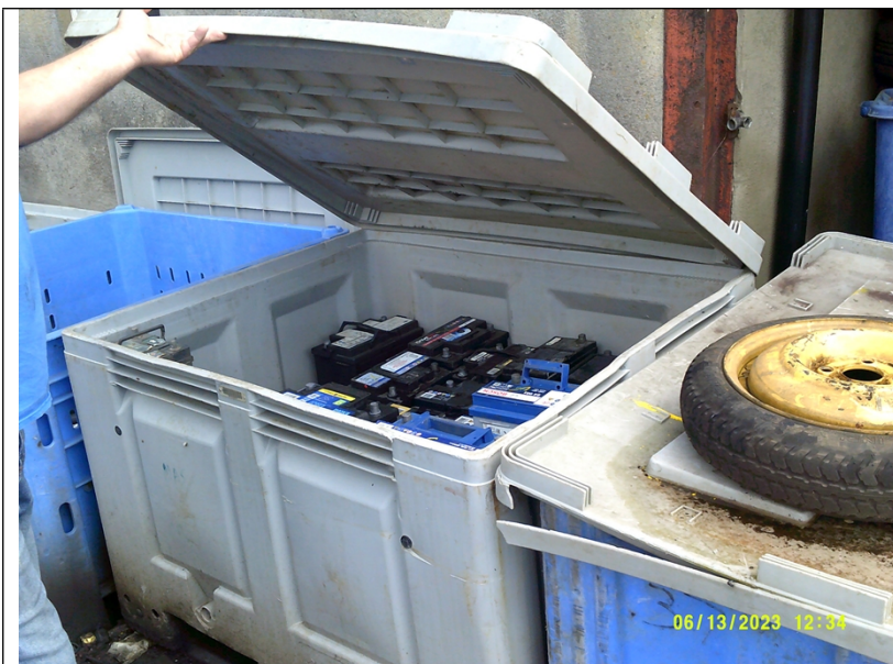
Figure 6: Acid resistant lidded container for waste batteries in depollution yard.
