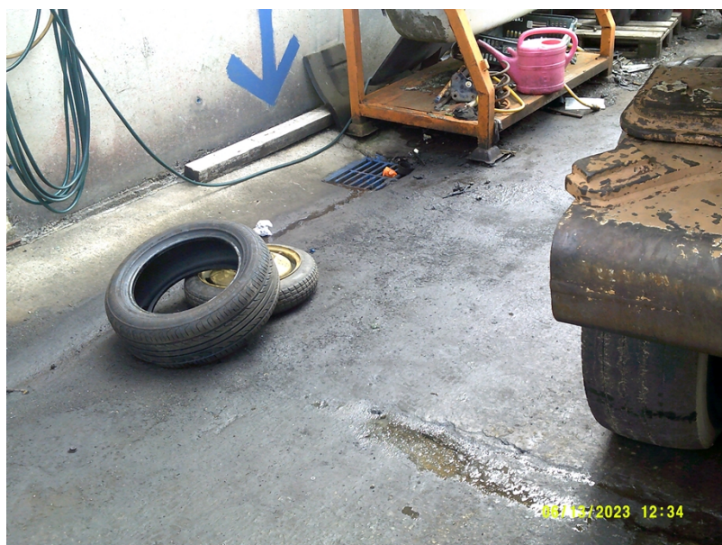
Figure 5: Oil in the depollution yard draining into closed drainage system.
