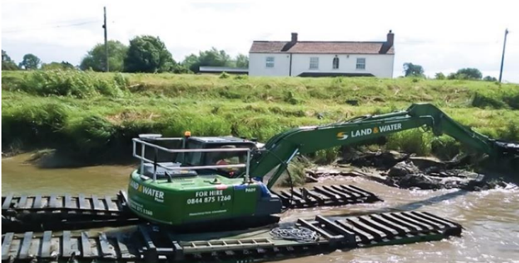
Typical example of Long Reach Amphibious Excavator
