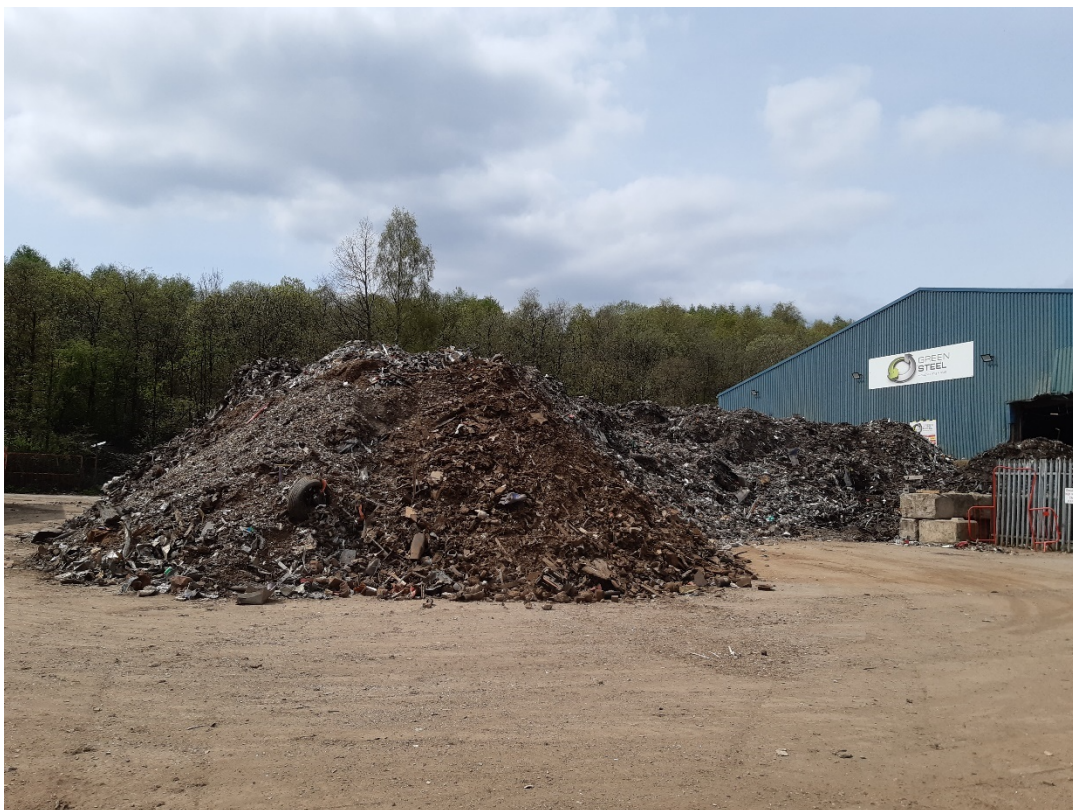
Photo 3 (above) stockpiles after staff used machinery to reduce height to less than 4m.
