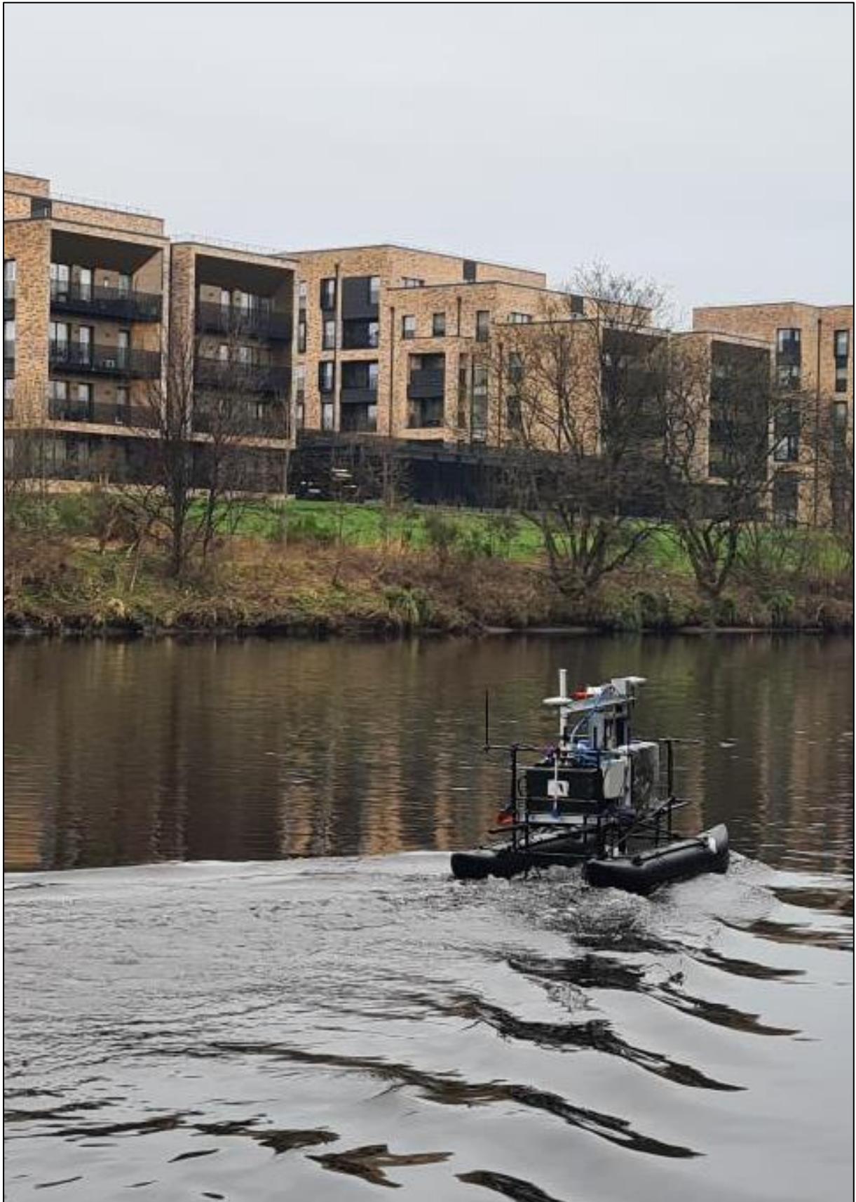
Figure 1.13 – Black Swan USV, performing a Network Rail Bridge Inspection in Glasgow
