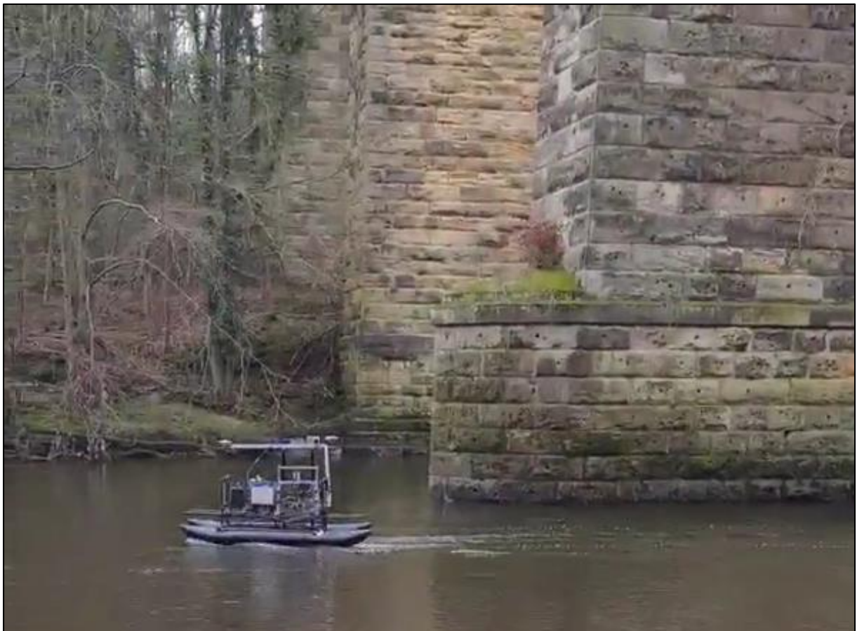
Figure 1.15 – Black Swan USV, performing a Network Rail Bridge Inspection in Motherwell
