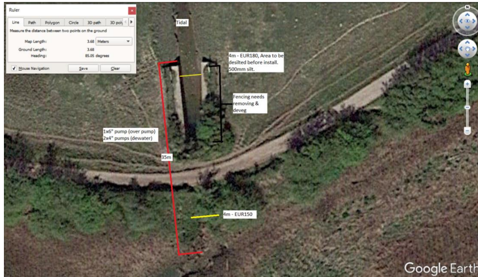
Picture 2 – Temporary Dams & Pumping arrangements
