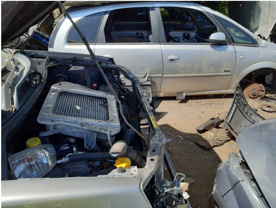
Photo 1 – vehicle with hazardous components remaining being stored on area of hardstanding.
