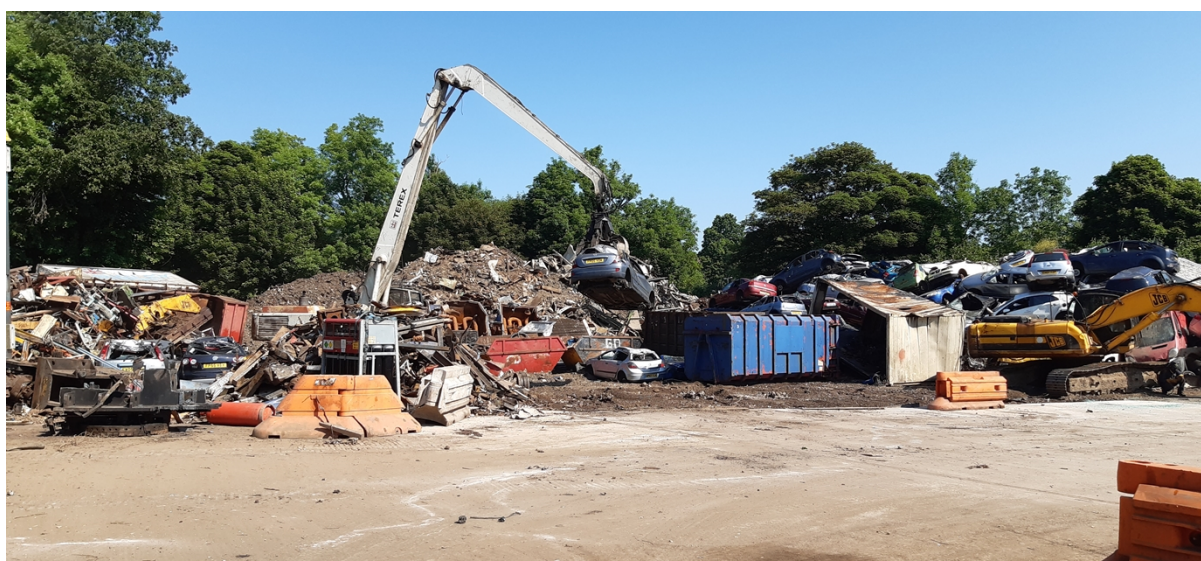
Photo 2 - Vehicle shells stored in unstable positions (background right)
