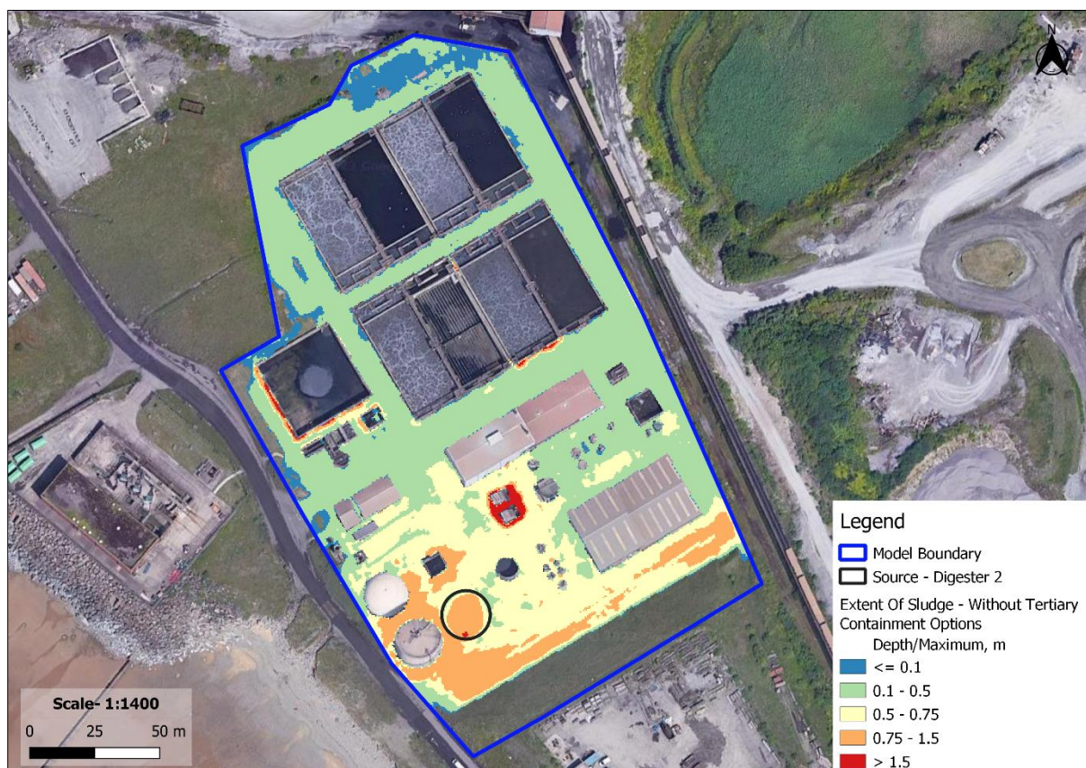
Figure 4.5: Sludge extent - Failure of Digester 2
