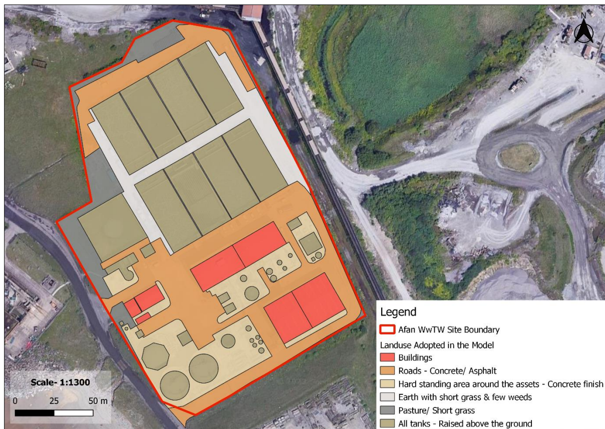
Figure 4.2: Different Surface types within WwTW
