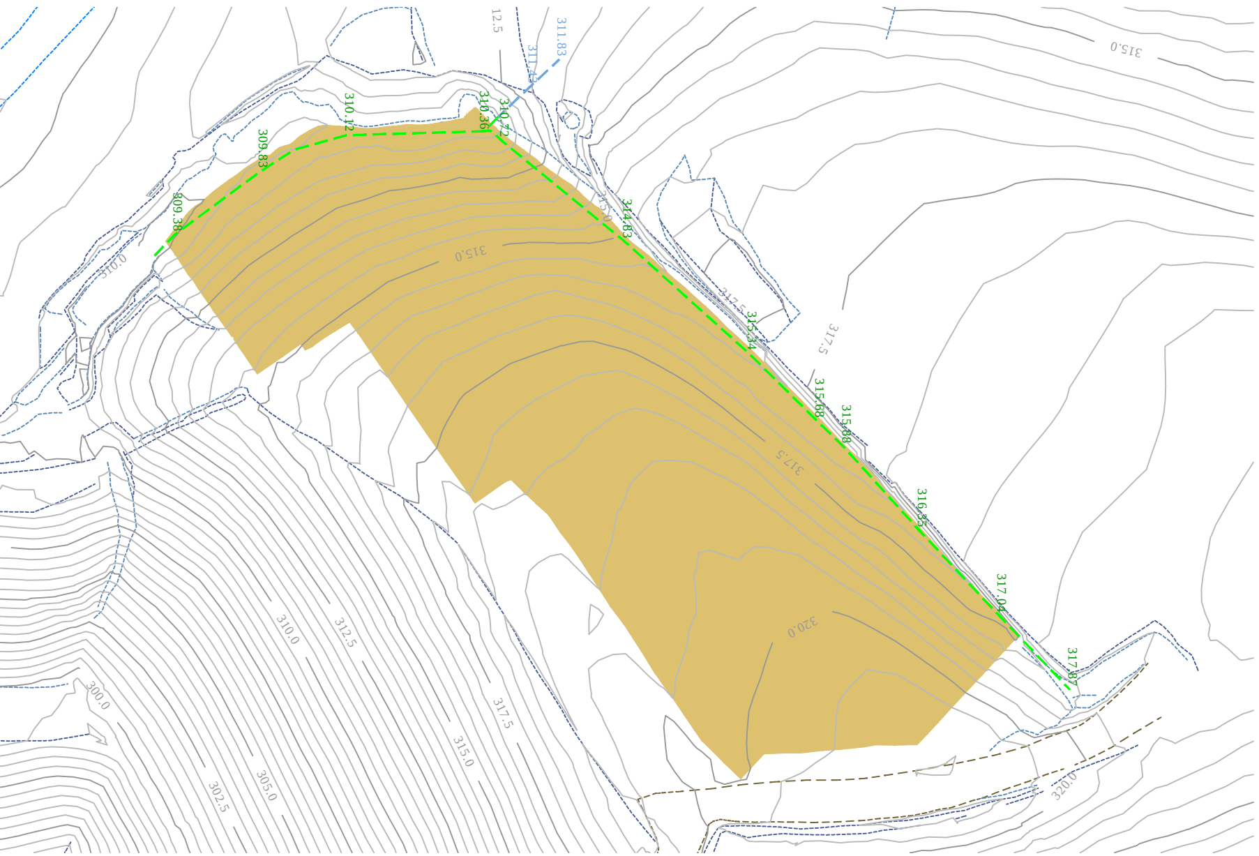
Figure 2 Regulating Layer and Leachate Drainage Pipework
