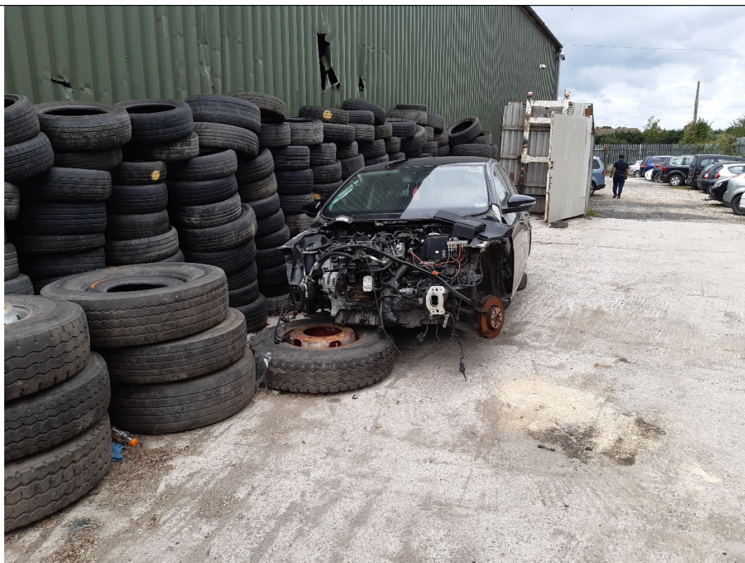
Photo 2 – Partially depolluted vehicle with hazardous components
