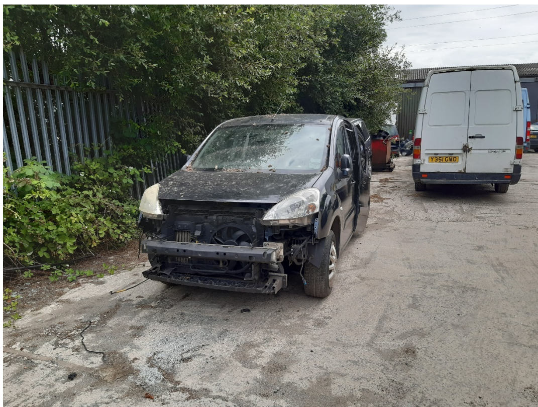
Photo 1 - Partially depolluted vehicle with hazardous components
