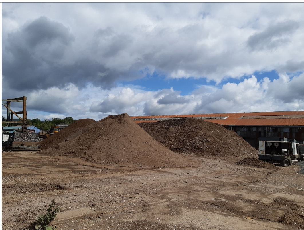
Photo 4 – stockpile behind 19 12 09 remains unprocessed fines (behind to the right)
