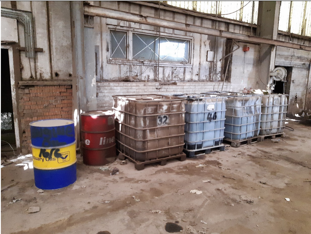
Photo 5 – IBC's and oil barrels stored without secondary containment in Unit 6
