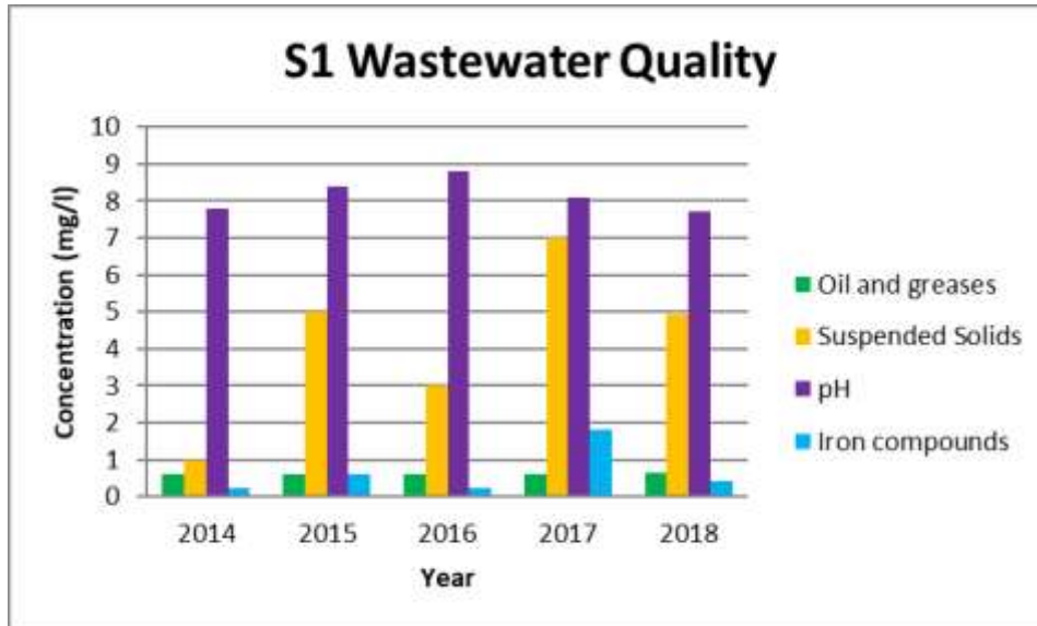
Figure 5: Melt Shop Waste Water Quality (mg/l)
