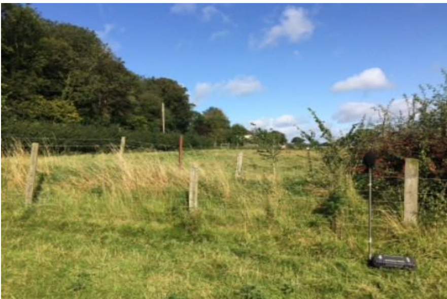
Figure A 1- Measurement Position 1 (1 of 3) - Sound level meter 1 - unattended
