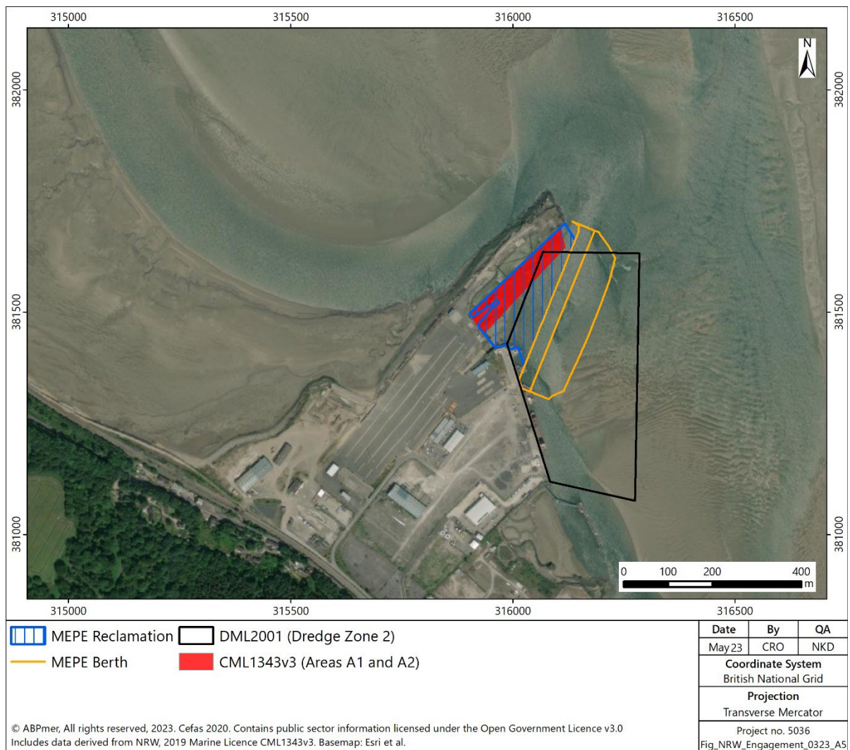
Figure 4. Existing permissions to remove and/or deposit materials within proposed MEPE reclamation and new berth
