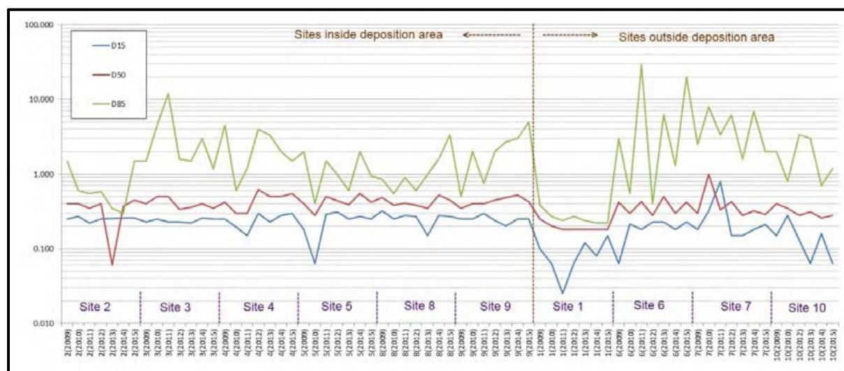
Image 5. Comparison of D15, D50 and D85 values for Mostyn Deep sediments (2009 to 2015)
