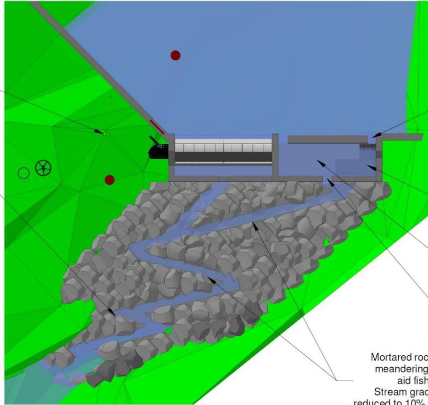
The meandering channel will create resting pools, upstream of protruding boulders, for fish swimming upstream
