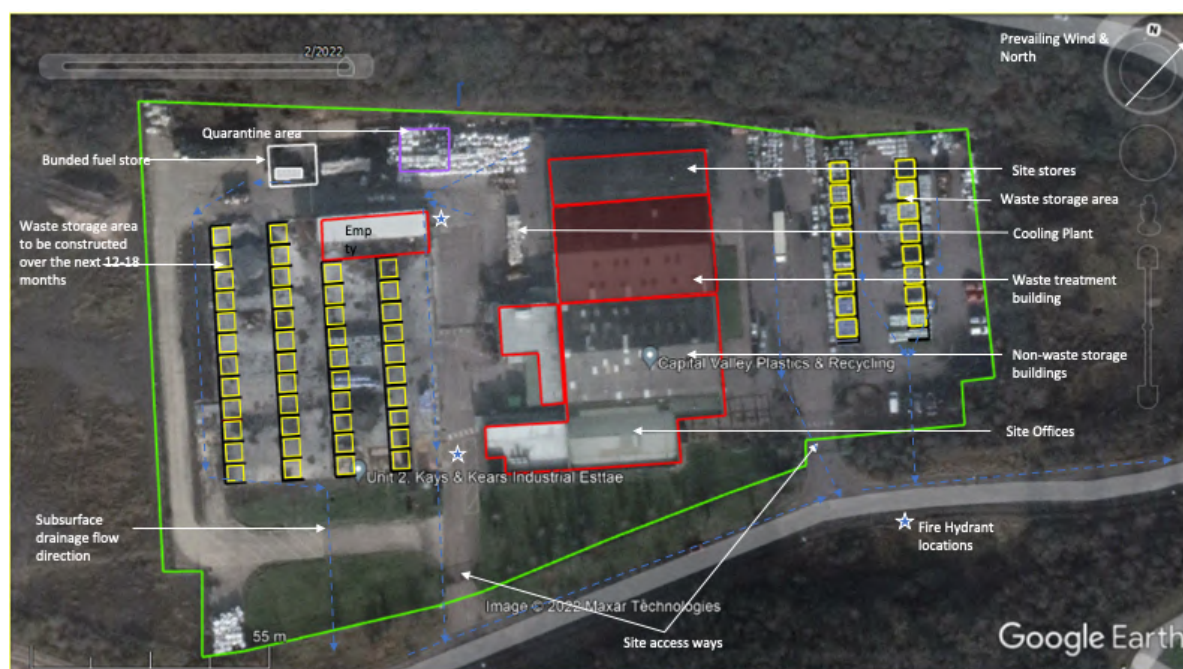
FIGURE 2: SITE PLAN - GENERAL LAYOUT AND FEATURES
