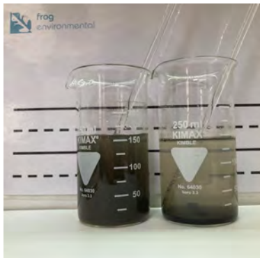
C. Test 3 Control vs WL 494 / 398 (further 15 second agitation from Test 2 plus 60 second settlement)
