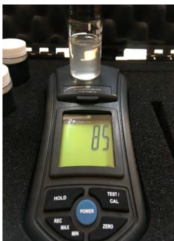
Figure 5: Turbidity meter
