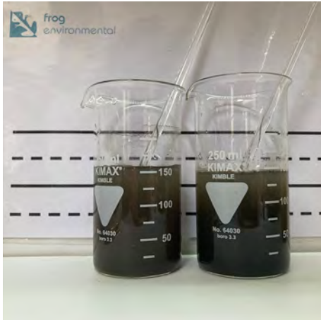
A. Test 1 Control vs WL 494 / 398 (15 seconds agitation plus 30 seconds settlement)
