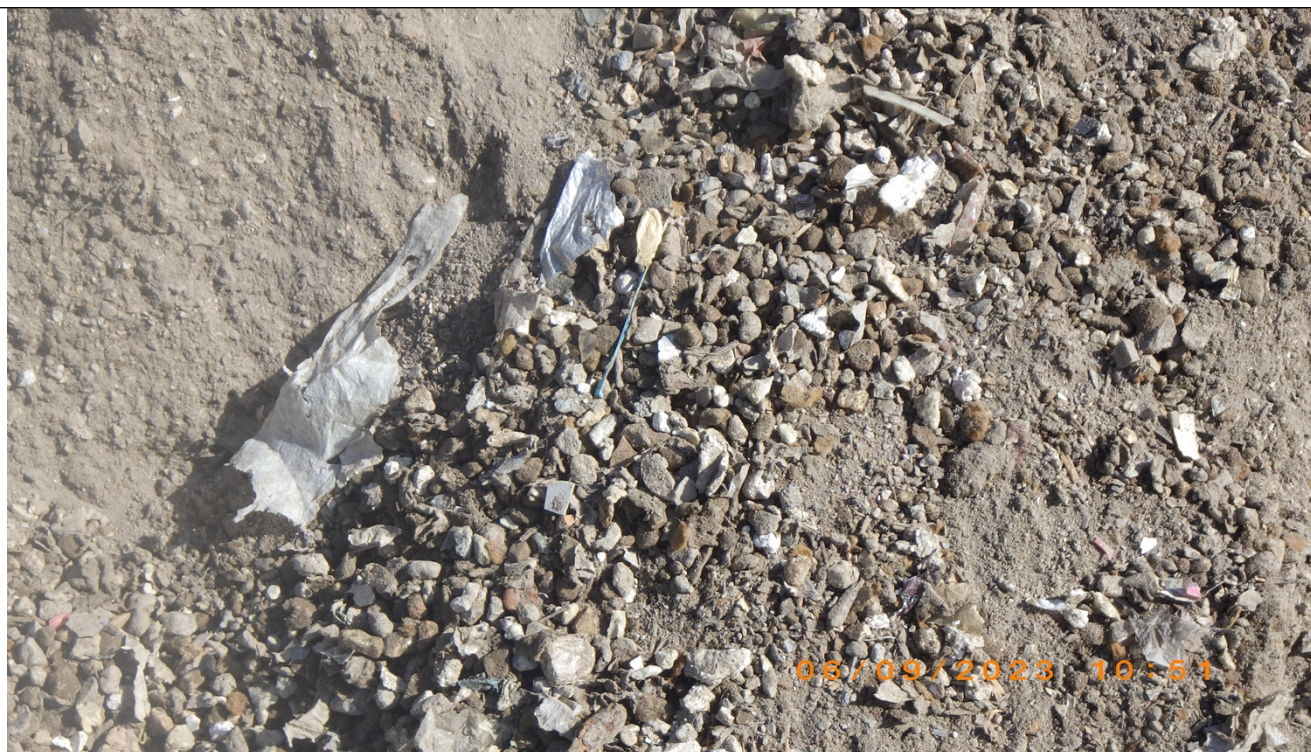
Photographs showing stockpiled soils / trommel fines
