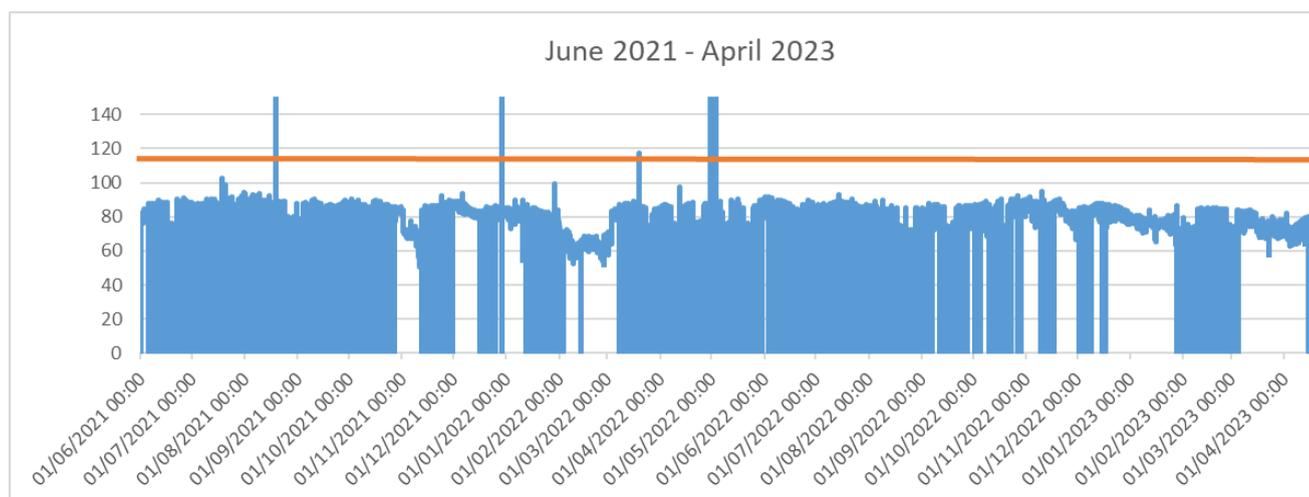
Pass forward flow (PFF) for this asset is 115l/s before the asset is permitted to discharge. during this period PFF never gets above 90l/s as such our calculations are based on 90l/s for PFF, this is at least 25l/s which was not being passed forward. The orange line in the above graph depicts the permit condition of 115l/s of PFF before the asset is permitted to discharge.
