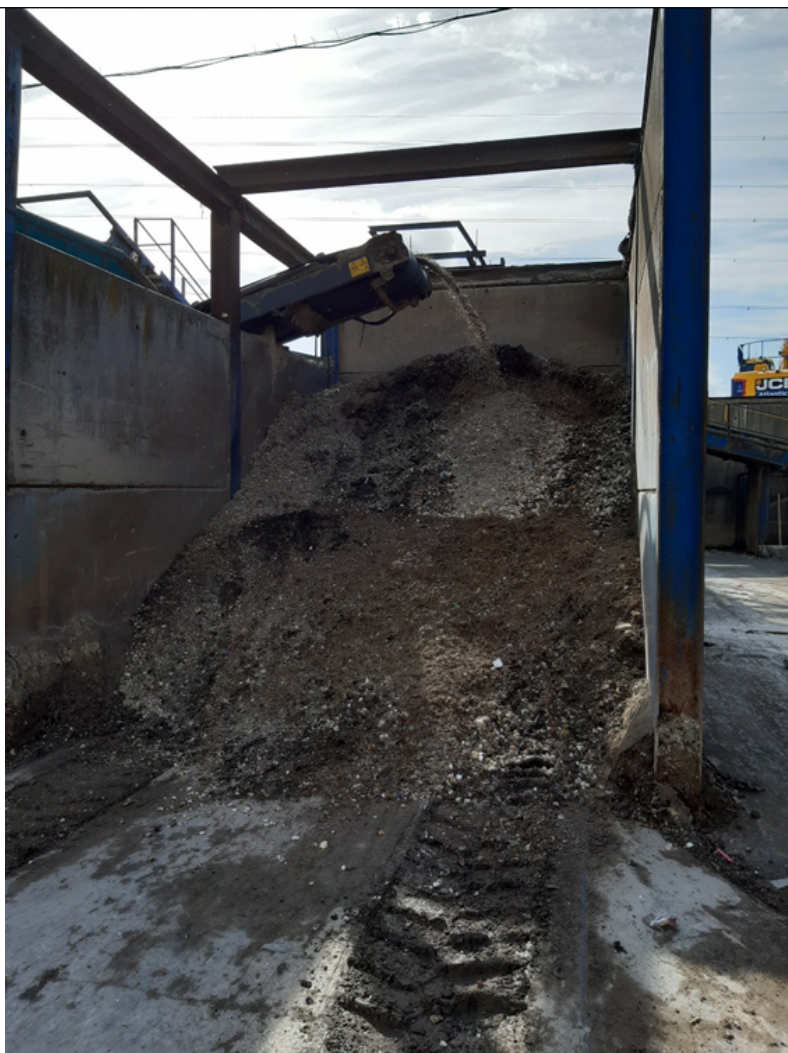
Picture 3 - SRF fractions being deposited into designated bay prior to mixing with imported SRF
