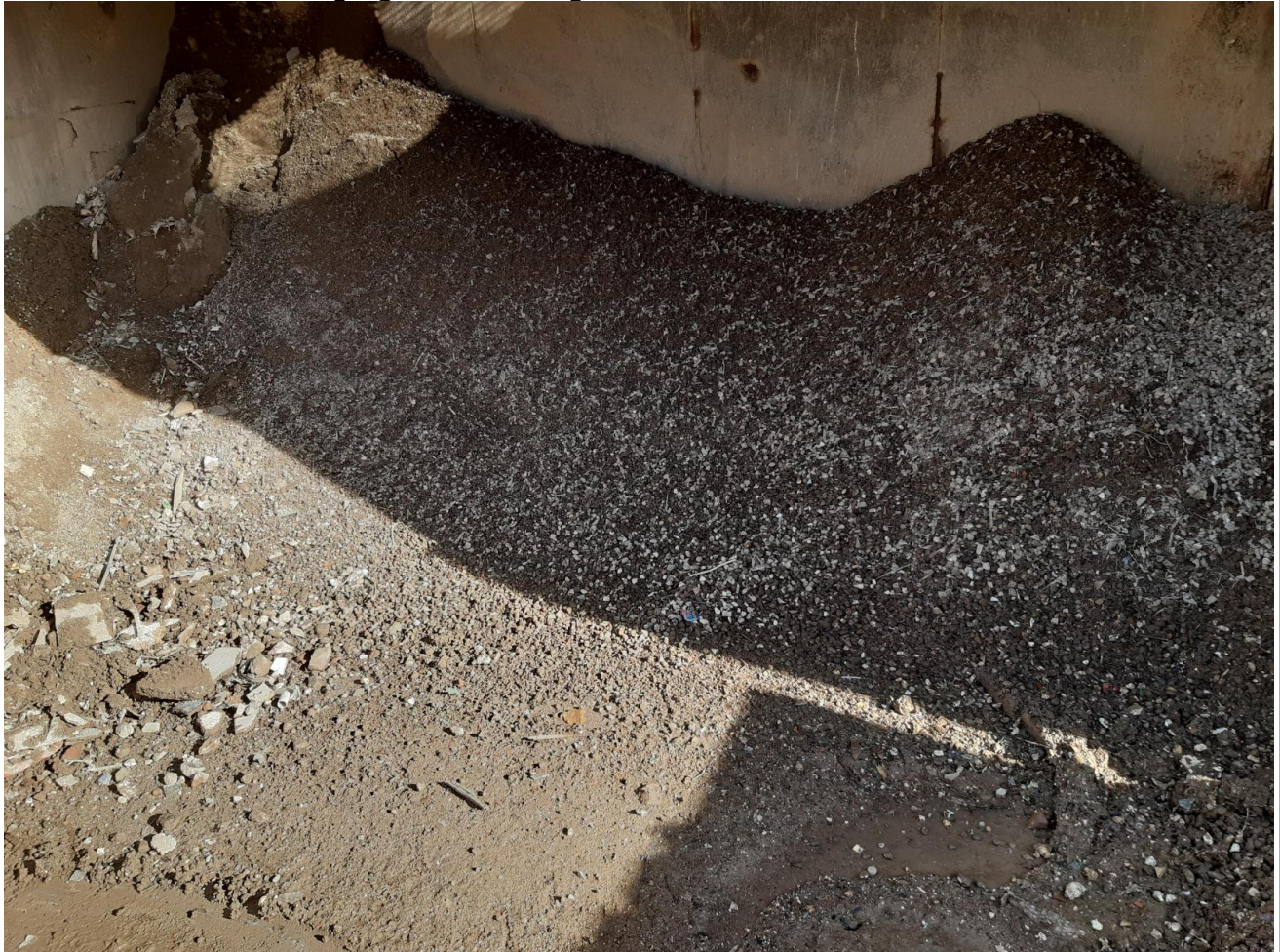
Photograph showing trommel fines on site, within a bay of the trommel.
