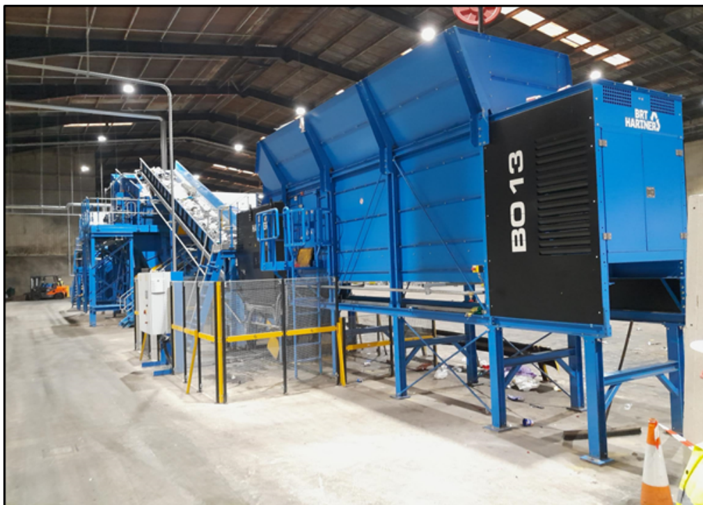
Image 2 – showing recycling machine; process sections: bag splitter, ballistic separator, picking line, and eddy current separator, taken at 11:07 on 25 October 2023
