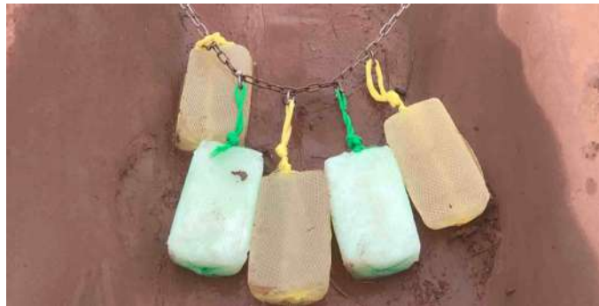
Photo 11 – The addition of Gel Flocculant in pipes
