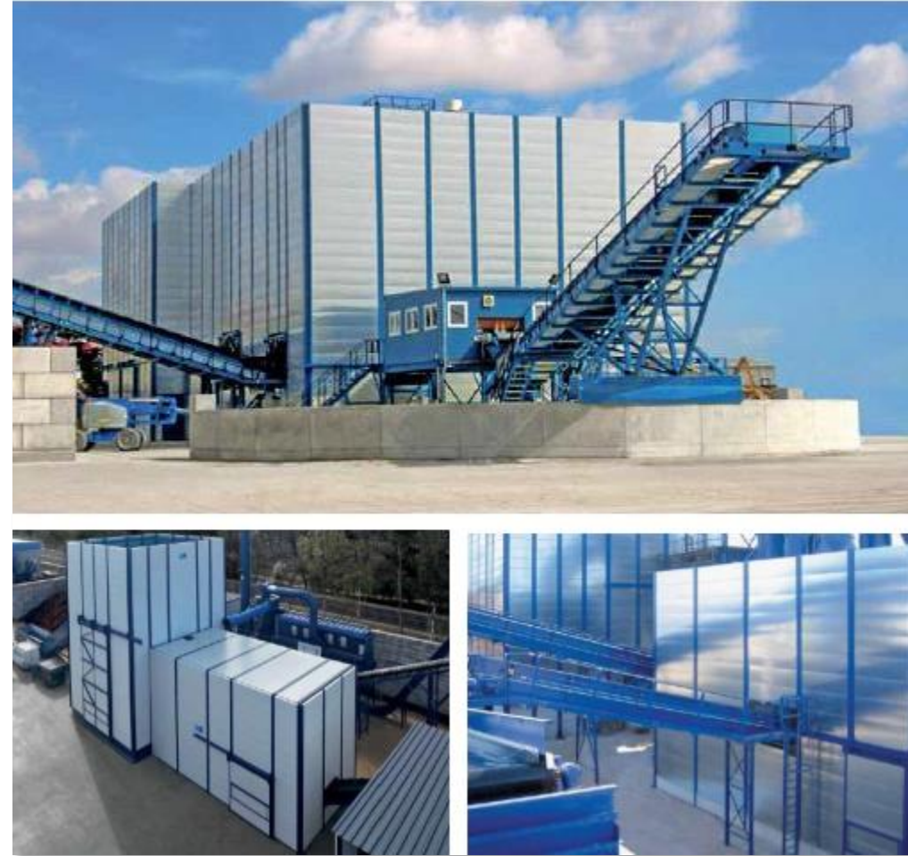
Figure 2: Typical scrap metal shredder (with noise abatement enclosures)
