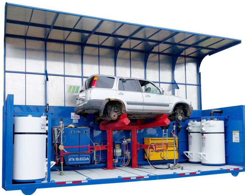
Photograph 5-1: Containerised ELV drainage system
